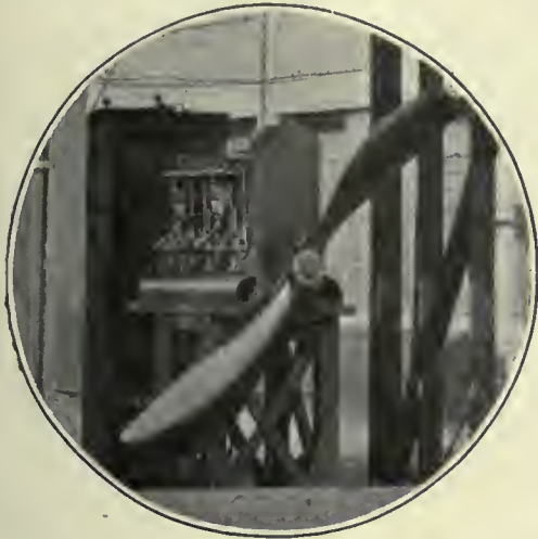
TESTING AN AEROPLANE ENGINE WITH PROPELLER.
