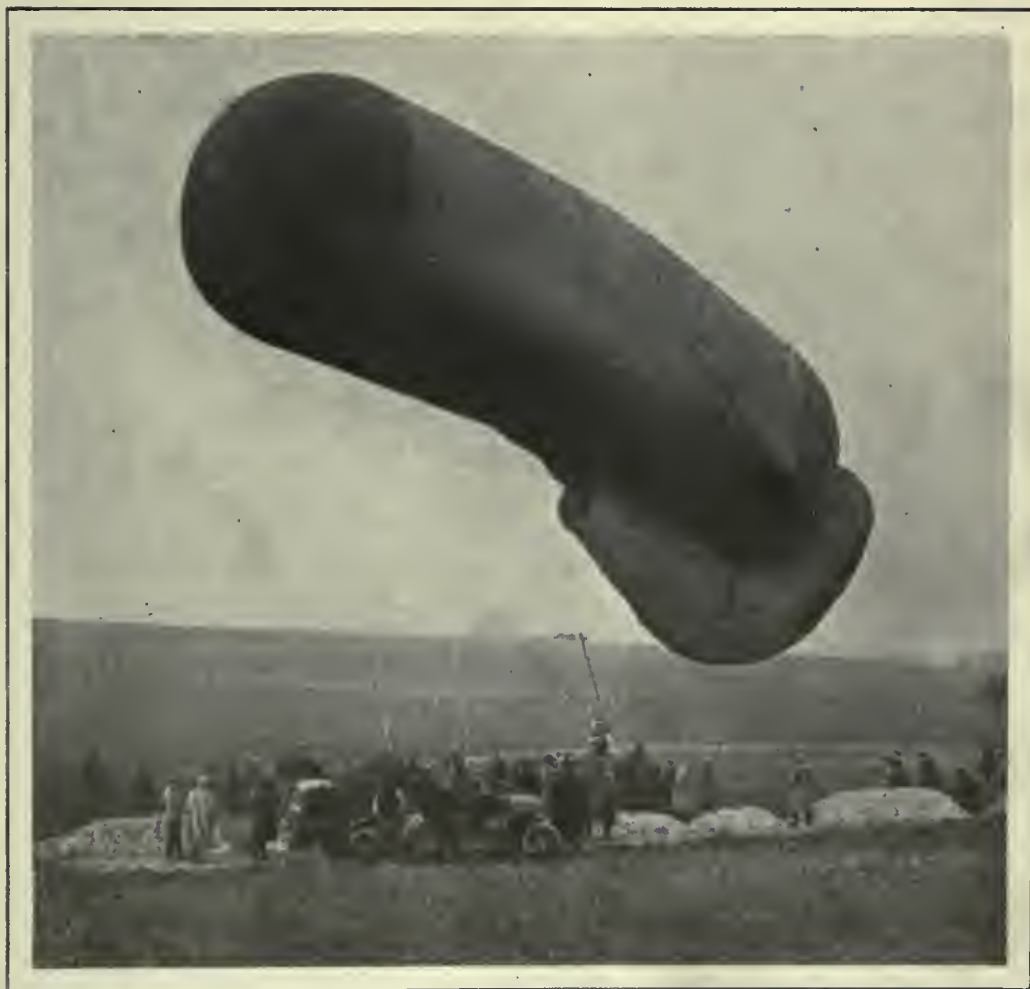
FRENCH OBSERVATION BALLOON AND ITS PORTABLE HAULAGE APPARATUS.
