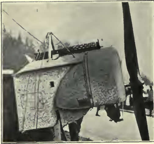
Showing arrangement of propeller and machine-gun.
